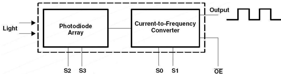
TCS3200D contains four types of filters: red filter, green filter, blue filter and clear with no filter. When the sensor is illuminated by a ray of light, the types of filters (blue, green, red, or clear) used by the device can be selected by two logic inputs, S2 and S3. Table 2 illustrates the relationship among S2, S3 and filter type.
